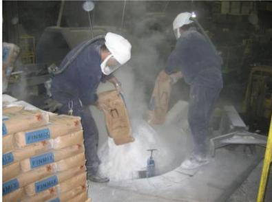
The process is completed by applying one of several types of vibration directly to the internal form causing the material to compact once installed in the annular area.
