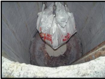
opening and dumping multiple bags of material onto the furnace bottom. Once the material is in place and evenly distributed, the bottom is ready for vibrating.
